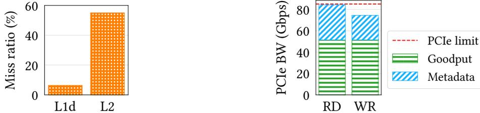
(a) Miss ratio for L1d and L2 caches. We observe 55% miss ratio for the L2 cache. (b) PCIe bandwidth utilization. Up to 39% of the read bandwidth is consumed with metadata.
